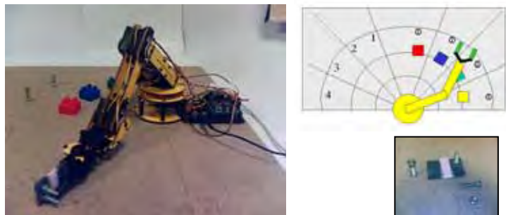
Fig. 3. Cooperative manipulation task scenario. User asks for screws from locations identified by color. While robot holds the plastic “table” (as illustrated) the user can insert the screws into the table (see inset).
