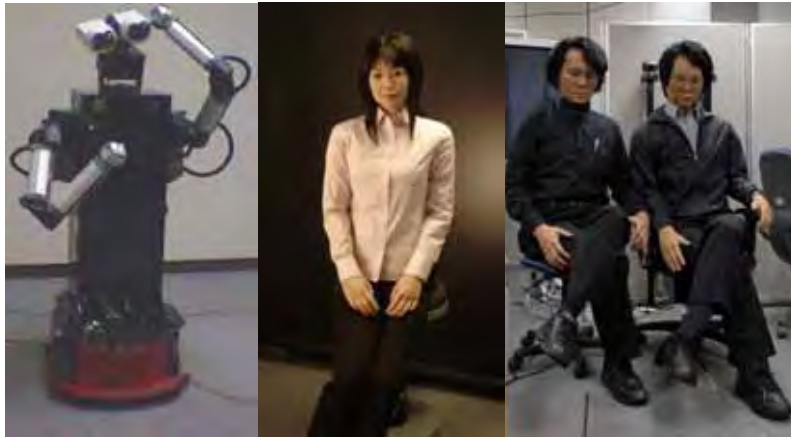
Fig. 1. Three categories of humanlike robots: humanoid robot Robovie II (left: developed by ATR Intelligent Robotics and Communication Laboratories), android Repliee Q2 (middle: developed by Osaka University and Kokoro corporation), geminoid HI-1 and its human source (right: developed by ATR Intelligent Robotics and Communication Laboratories).
