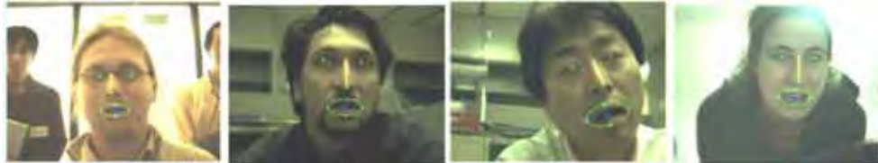
Fig. 6. Screen capture of tracked outer lip contours for various skin tone colors and different lighting conditions.
