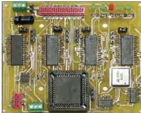
Fig. 21. The prototype custom embedded real-time controller. The board has dimensions of 69 \times 85\text{mm}^2 .
