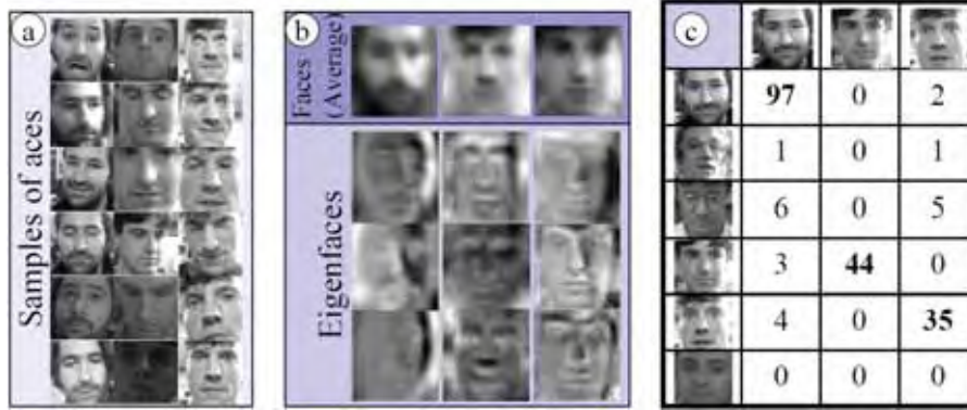
Fig. 9. a) Face image samples are shown for each of three people out of a database of six; b) Average face image for three people on the database, together with three eigenfaces for each one; c) Confusion table with face recognition results.
