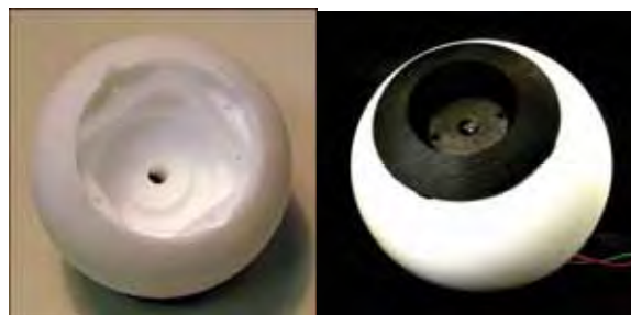
Fig. 8. The machined eye-ball (left), and the assembled eye-ball (camera cables shown in background).
