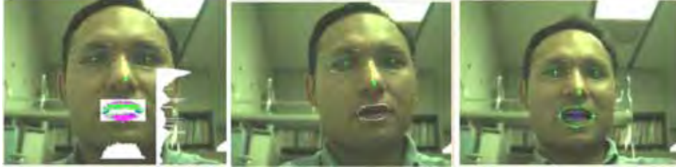
Fig. 3. Left image: result of the Bayes decision rule, its vertical projection (bottom) and integral projection of intensity plane between nose and chin (right). Middle image: estimated outer lip contour using the result of the Bayes rule. Right image: a parameterized outer lip contour.
