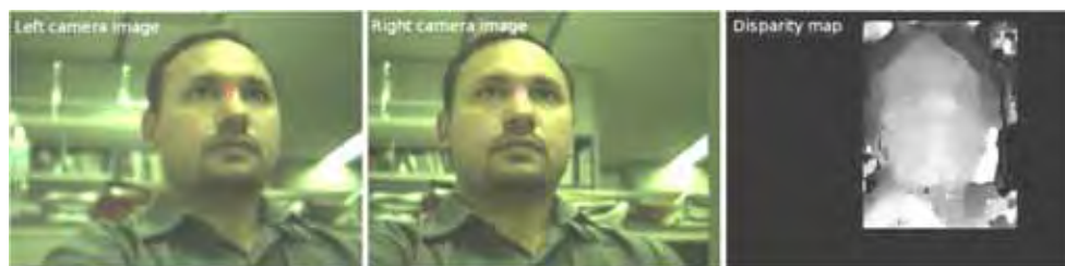
Fig. 7. Screen capture of the left and right camera images, and their disparity map around the face region of interest.
