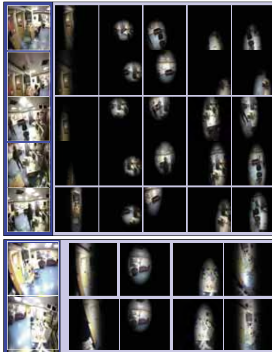
Fig. 13. Localizing and recognizing objects from contextual cues. (top) Samples of scene images are shown on the first column. The next five columns show probable locations based on context for finding a door, the smaller sofa, the bigger sofa, the table and the chair, respectively. Even if the object is not visible or present, the system estimates the places at which there is a high probability of finding such object. Two such examples are shown for the chair. Occlusion by humans do not change significantly the context. (bottom) Results in another day, with different lightning conditions.
